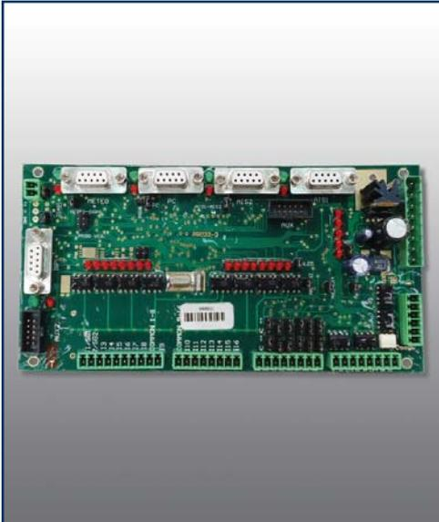
The MMB 02 daughter board is a universal device especially designed for aids-to-navigation equipment monitoring, in particular lighthouses and beacons. Due its versatility, it is ideal for offshore platforms, since all the aids to navigation can be controlled by it.
