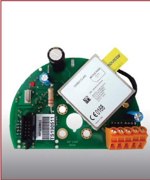
MFGSM circuits are small and compact remote monitoring devices, fitted inside our LED lanterns. The sending and receiving remote control signals is done through GSM mobile phone messages.
