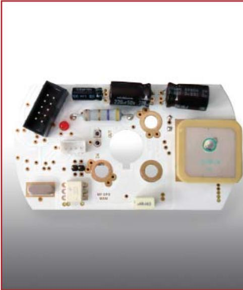
MFGPS position and synchronisation module is a device with double function. On the one hand, it is used to determine buoy positioning and, on the other hand, to synchronise lanterns through a GPS receiver of 12 channels.
